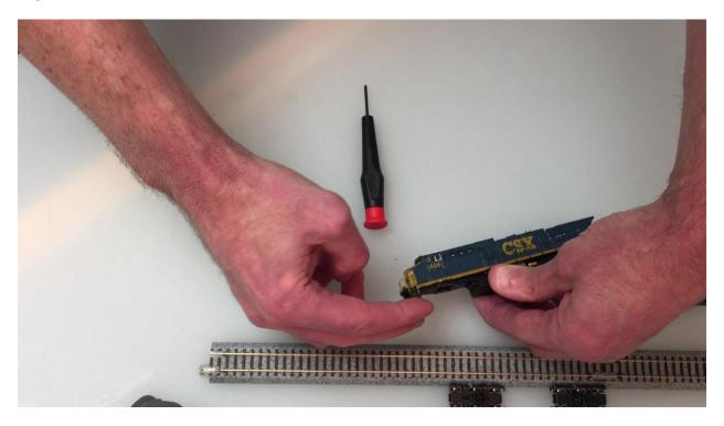
Step 6: Lift the shell away from the chassis, be aware of the cab light wires and do not pull it too far away.
