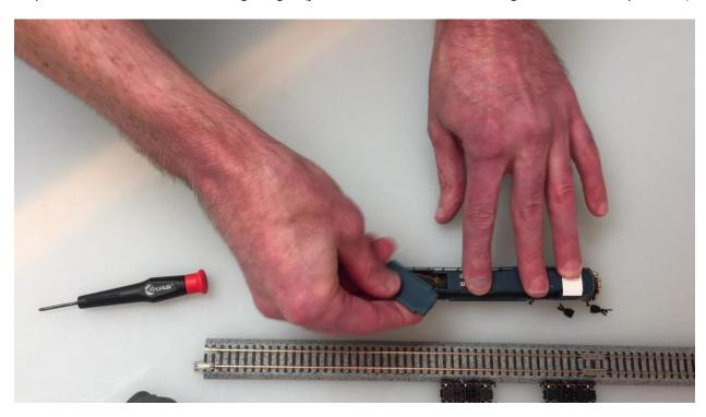
Step 4: Push down on the chassis while pulling up under the steps on the rear of the engine.
