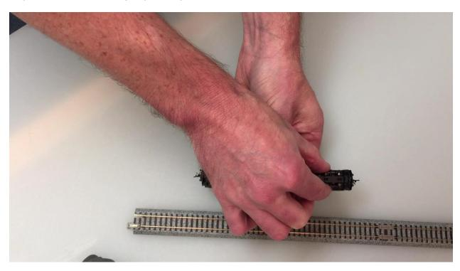
Step 2: Remove the couplers on either end (1 small Philips head screw to remove for each coupler).
